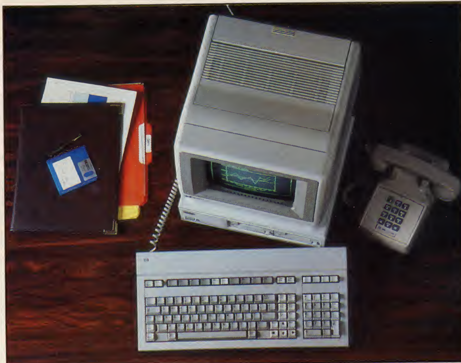
The HP 150 has a relatively compact footprint (11 x 13") compared to the IBM PC (16 x 20"). On the other hand, the keyboard is a largish 18 x 9".
